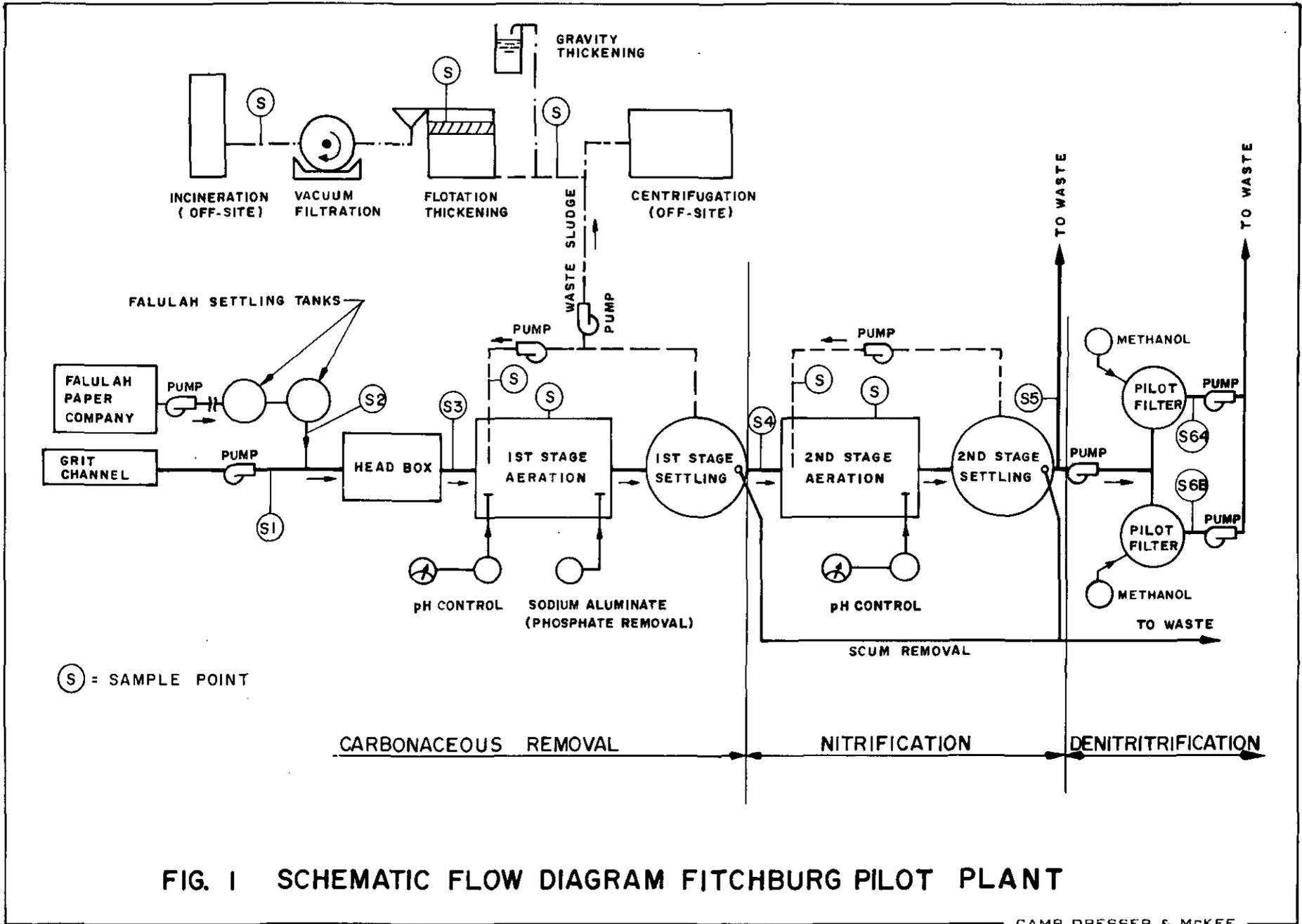
FIG. 1 SCHEMATIC FLOW DIAGRAM FITCHBURG PILOT PLANT
