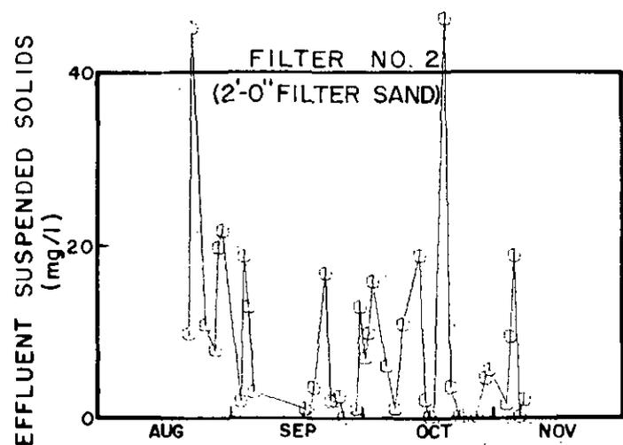
FIG. 29-SUSPENDED SOLIDS REMOVAL IN PILOT FILTERS
