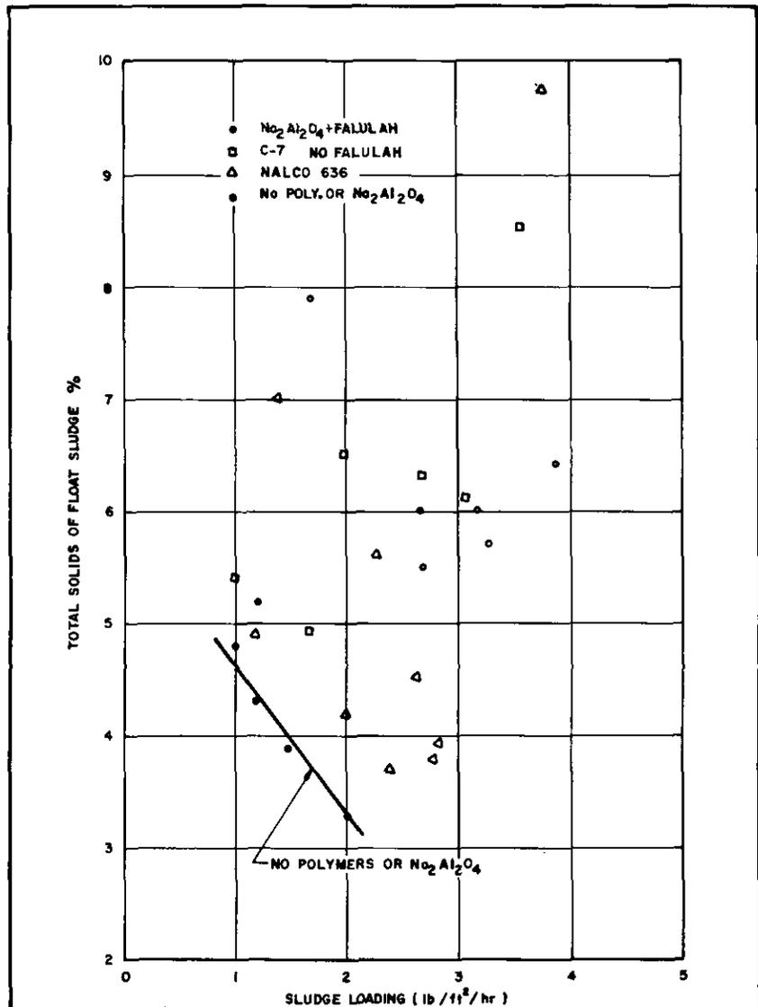
FIG. 26 EFFECT OF SLUDGE LOADING RATE ON SLUDGE THICKENING
