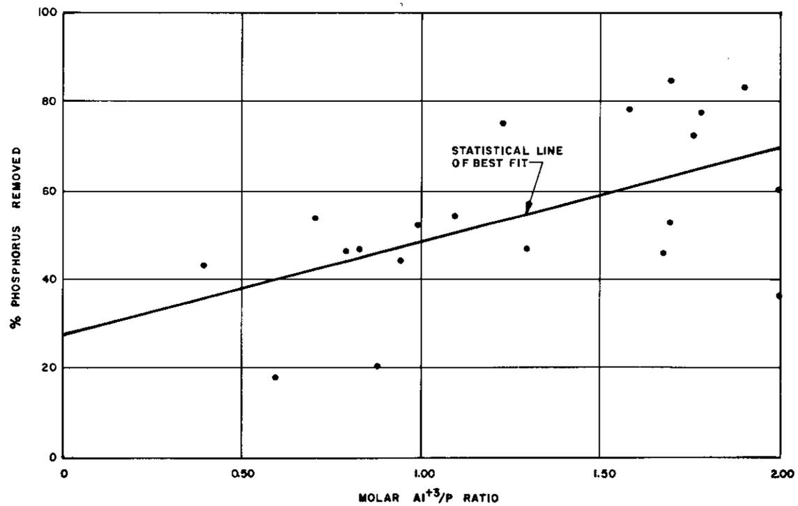
FIG.23 EFFECT OF DOSAGE OF ALUMINUM ON PHOSPHORUS REMOVAL
