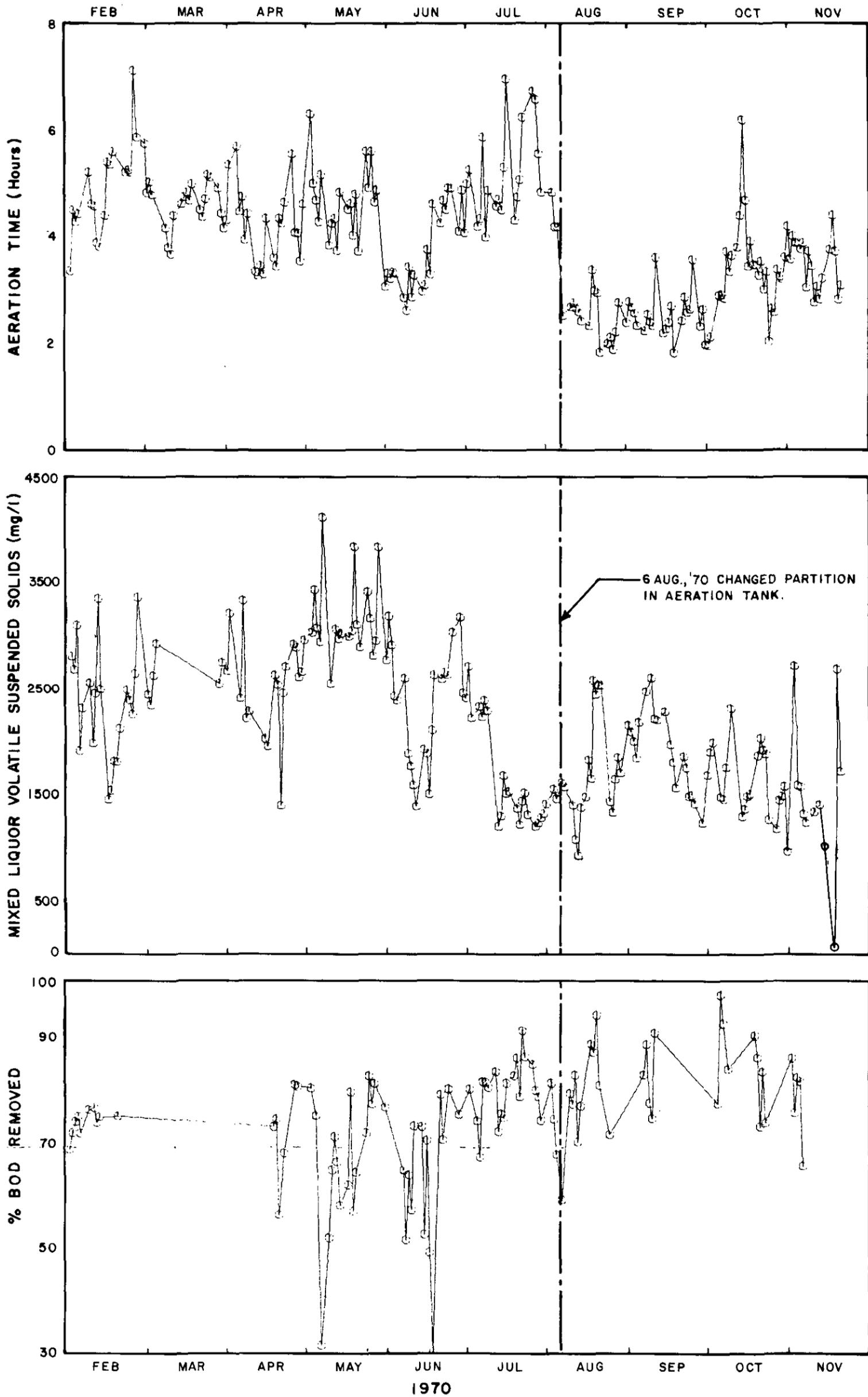
FIG. 6 DAILY VARIATION OF 1ST STAGE % BOD REMOVED, MLVSS AND AERATION TIME
