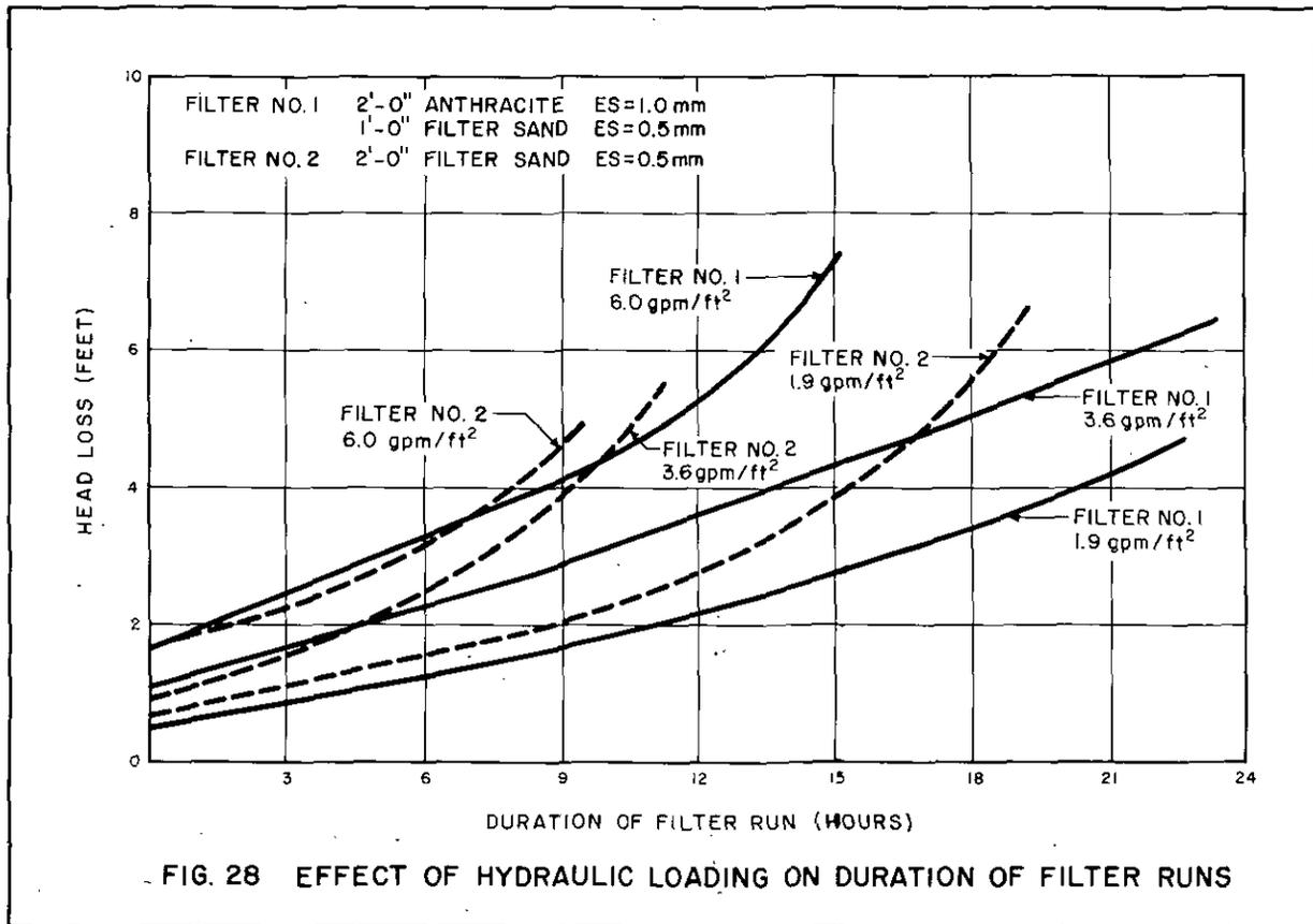
hours. Backwashing of filters was done daily. It is significant to note (Figure 28), that the rate of increase of headloss was consistently higher for Filter No. 2 than the rate of increase for Filter No. 1. This may be attributable to the fact that Filter No. 2 had more than twice the height of filter sand than Filter No. 1.
