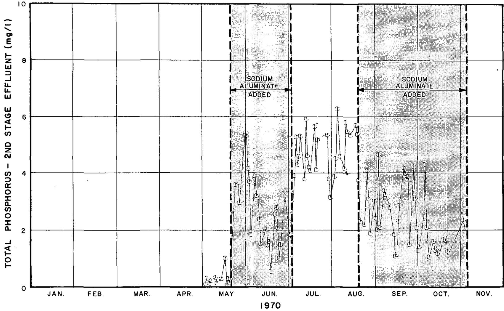
FIG.24 EFFECT OF SODIUM ALUMINATE ON PHOSPHORUS CONCENTRATION
