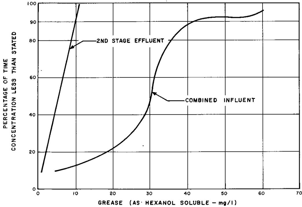
FIG. 11 PILOT PLANT RESULTS 22 APR. TO 20 NOV., 1970
