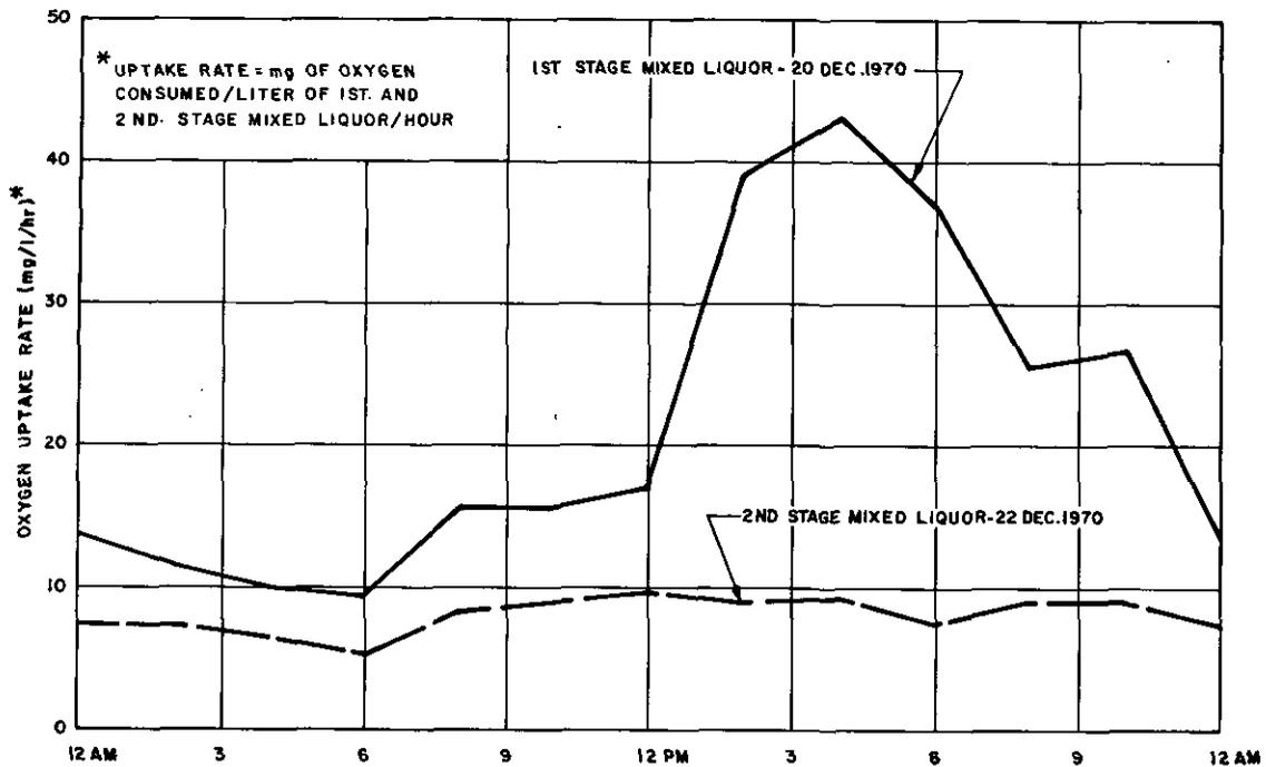
FIG. 19 DIURNAL VARIATION OF OXYGEN UPTAKE RATES OF 1ST & 2ND STAGE MIXED LIQUOR
