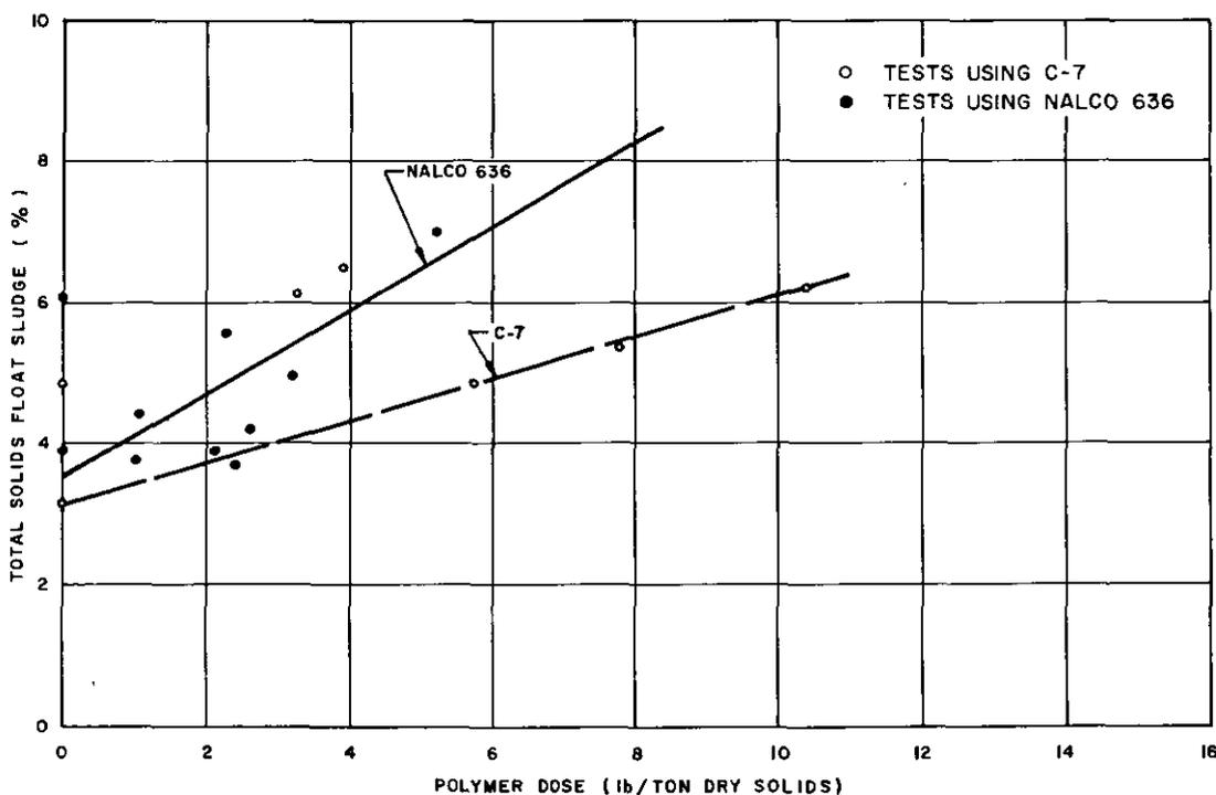
FIG. 25 EFFECT OF POLYMER DOSE ON SLUDGE THICKENING
